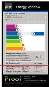
Thermal Transmittance (U window) 1.3 W/m<sup>2</sup>.K
